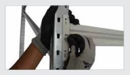
Click the remaining beams into place and attach the locking pins
